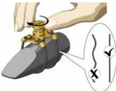
3. Finally disassemble the ligature and reassemble it as desired, complete with reed ("Ligature assembly" pages 9-10).
